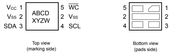
Figure 2. 5-pin package connection
